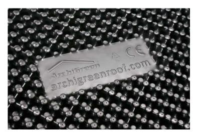
SedumDrain® 25 is the result of extensive research and testing in the quest for the optimal water reservoir and drainage layer for green roofs. The outcome is an unmatched 25 mm high, lightweight water retention and multi-level drainage board, manufactured from recycled high impact polystyrene (HIPS) and is black in colour. The surface is thermoformed on both sides with unrivalled centralised perforations on the top.
